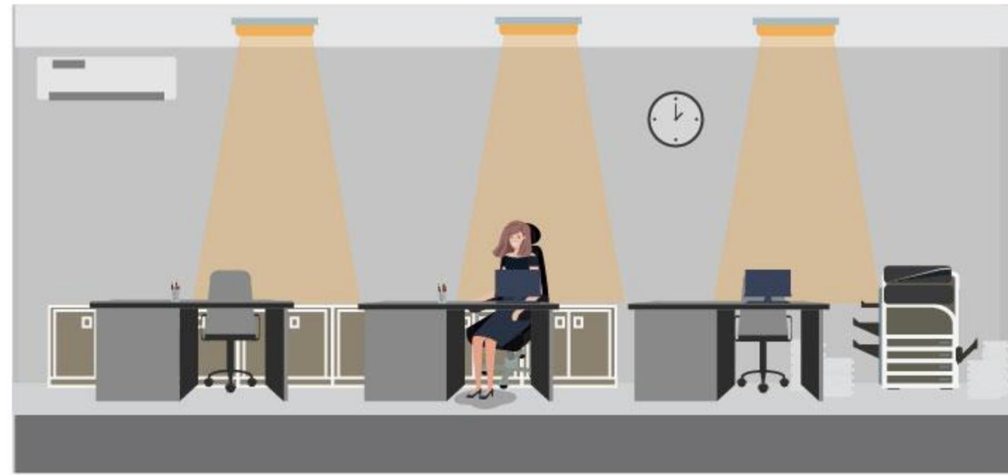
When the sensor detects a moving object, the light automatically lights up and enters the set delay time.
