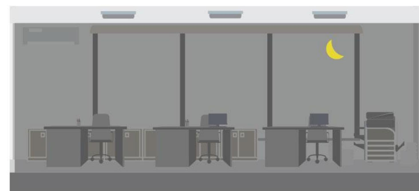
The light goes out automatically after the preset delay time has elapsed when the moving object leaves.
